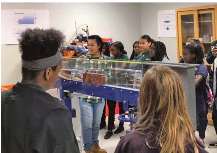
Figure 2. Students observing hydraulic jumps in an open-channel flume
