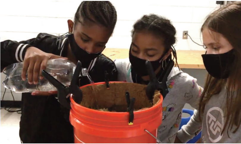
Students measure the infiltration rate of water flowing through a mixture of sand, gravel, mch, and soil.
